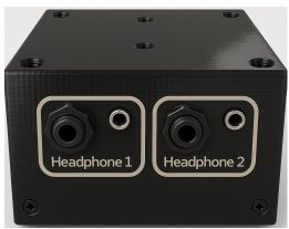
The Simon Systems CB-2 allows two pairs of stereo or mono headphones to be driven from the same audio power amplifier. Each output has a both ¼" and 1/8" stereo (or mono) jacks, and is controlled by a custom-made high-quality stereo volume control. These power rated potentiometers, are made with noise-free conductive plastic, and therefore provide superior performance to wirewound potentiometers.
